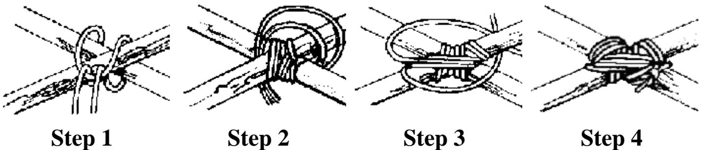
1. A lashing used in lightweight construction work.
