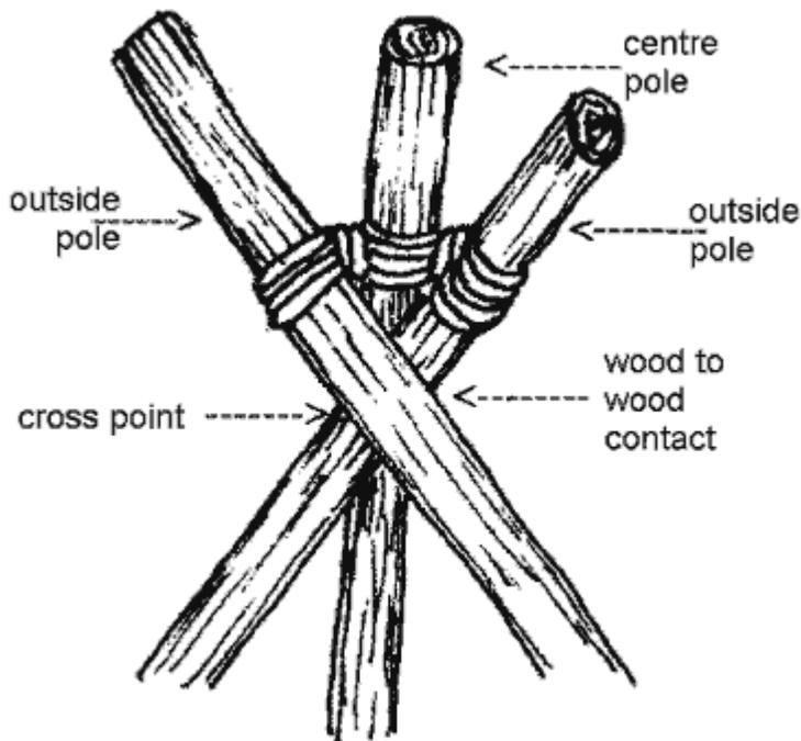
Set up the tripod by crossing the outside poles so that the cross point of the poles is under the center pole. Crossing the outside poles under the center pole causes part of the load that is placed on the tripod to be taken up by the wood to wood contact of the poles.
