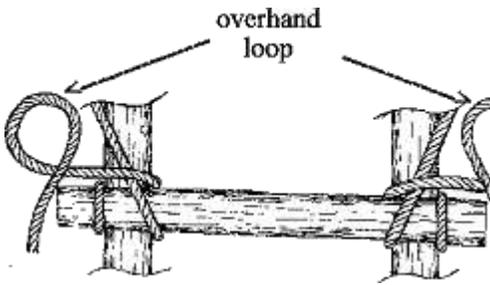
**Step 5:** Then pull the loop over the end of the rung.
