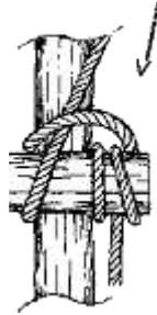
**Step 6:** Work each rope until it is tightened around the rung and the rung is in its desired position.
