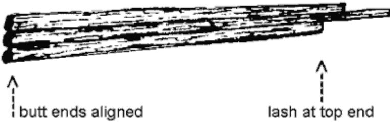
For most tripod lashings, lay the pole side by side with the butt ends aligned. The alignment of the butts of the pole insures that the tripod legs are the desired length
