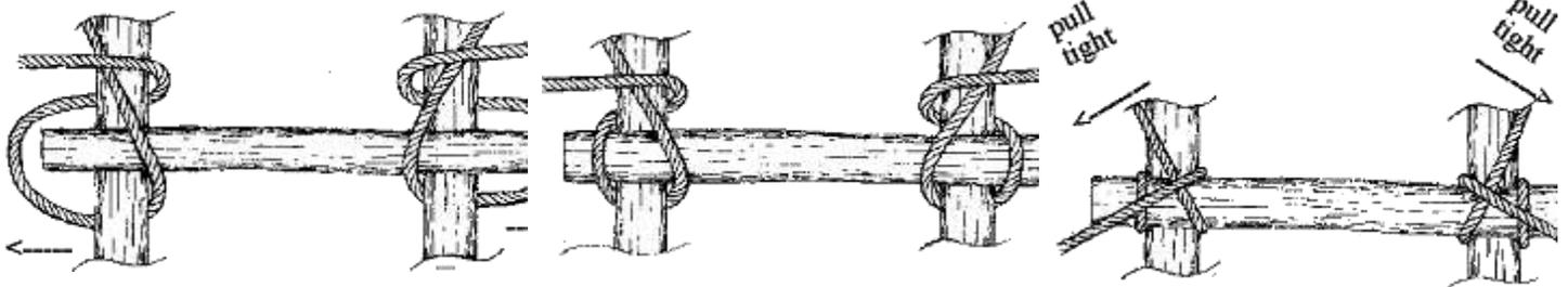
**Step 4:** Pull the running part side of each overhand loop behind and to the outside of each rail.
