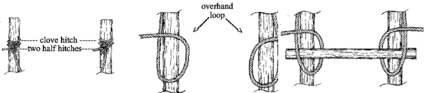
**Step 1:** The ladder lashing is started by using a clove hitch stopped with two half hitches to secure a rope to the top end of each rail.
